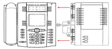
The M675i provides 10 softkeys in each column (totaling 20 keys) on the keypad. The M675i also provides 3 keys at the bottom left of the unit. These keys represent "Page 1", "Page 2", and "Page 3" of the LCD display. The M675i has 20 keys available on each page (totaling 60 softkeys). Each key provides an LED for indicating call status. The M675i provides an LCD for displaying key labels.
