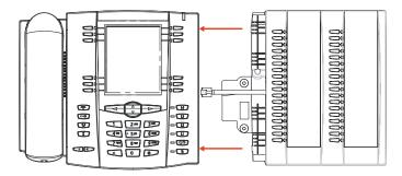
The M670i provides 18 softkeys in each column (totaling 36 keys) on the keypad. Each key provides an LED for indicating call status. The M670i provides a paper label for convenient key labeling.
